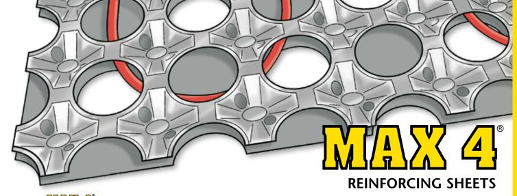
Reinforcing sheets are manufactured from 2 sheets of special profiled steel and designed for use on existing timber or concrete floors where an extremely thin liquid screed solution is required. MAX 4<sup>®</sup> reinforcements sheets are available in two variations - FS10 -10 mm thick and FS20 -20 mm thick and both ideal for use with under floor heating.
